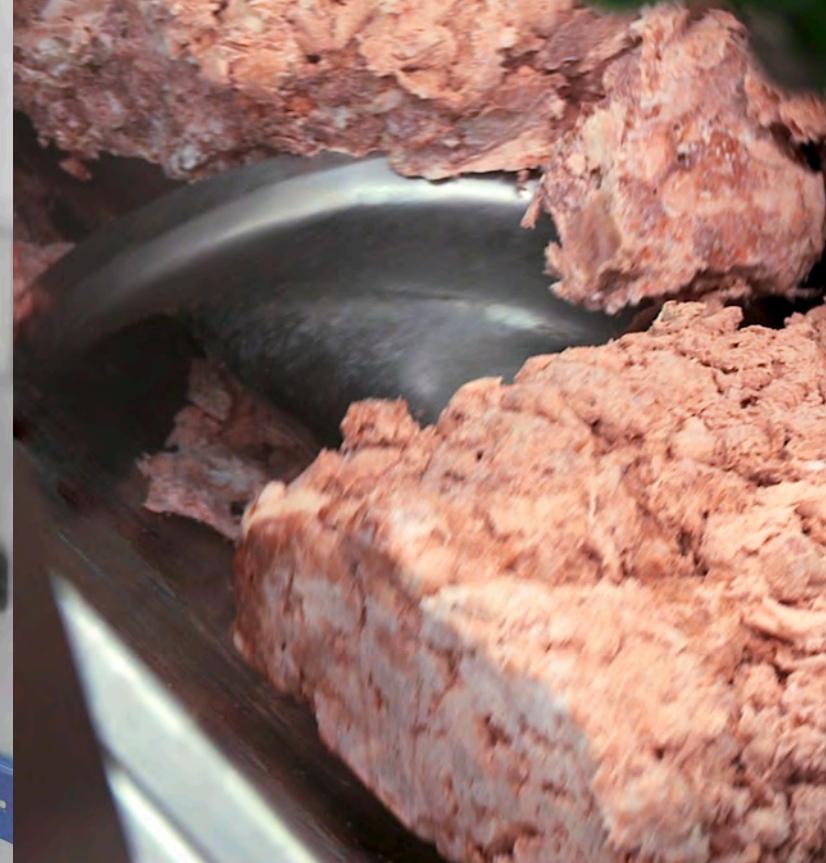
Feeder worm made from special cast iron with skinning edge
