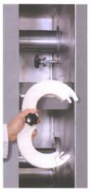
The front bearing of the mixing shaft can be removed easily. The mixing shaft of the mixer M 200 can be quickly and easily dismantled for cleaning purposes. With mixer M 500, the seal of the mixing shaft to the drive shaft can be easily flapped open and dismantled. The mixing and transport worm for both mixers can be pulled out at the front after the emptying flap has been opened and the protective cover swung away.
