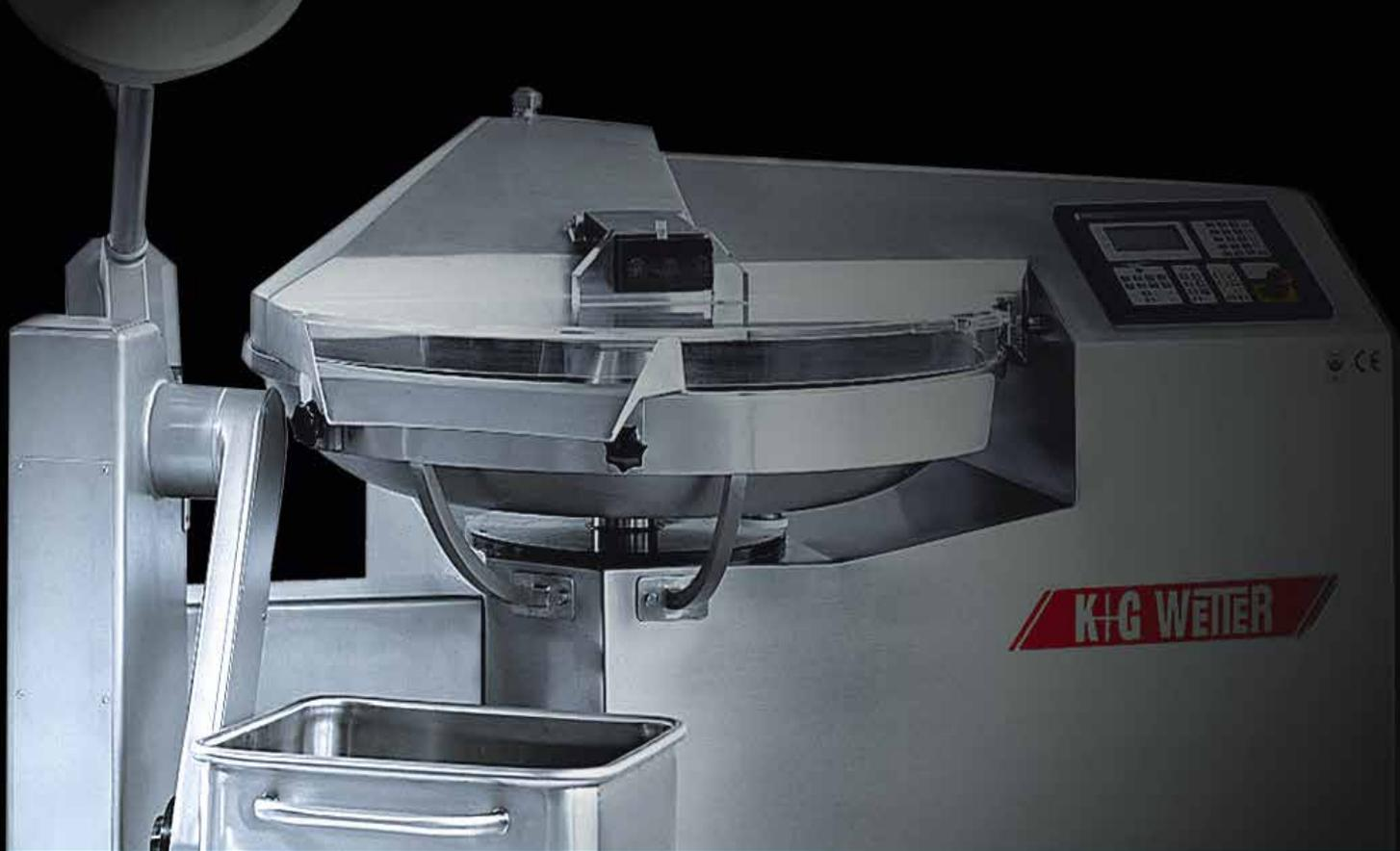
Depending on model, the bowl drive offers two speeds or is infinitely adjustable for the benefit of lower energy consumption and lower start-up current peaks. The STL design also offers a serial limit deactivation for temperature, bowl rounds and time.
