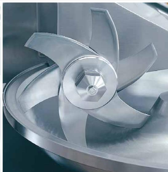
Fine sausage meat knife head with six knives that cut and emulsify extremely fine boiled sausage meat. Mainly for high-speed bowl cutters with infinitely adjustable drive and knife system that can be balanced out. The number/setup of the knives can be varied.
