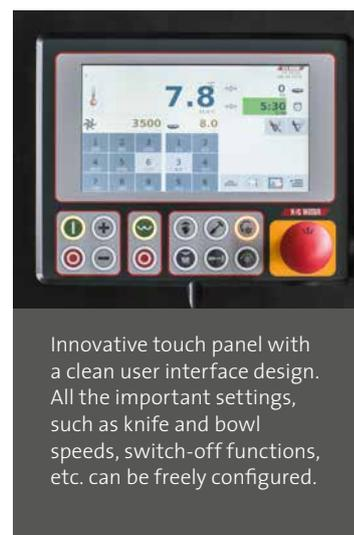
Innovative touch panel with a clean user interface design. All the important settings, such as knife and bowl speeds, switch-off functions, etc. can be freely configured.
